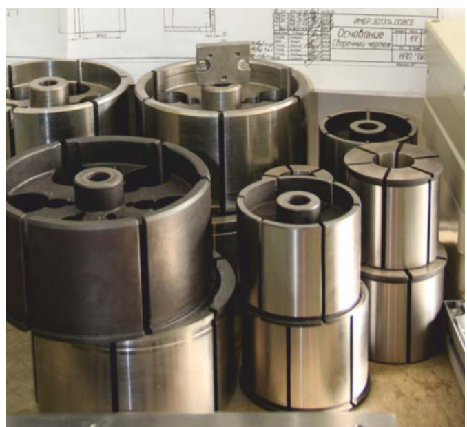
Collets for fixing bearings on the stand
