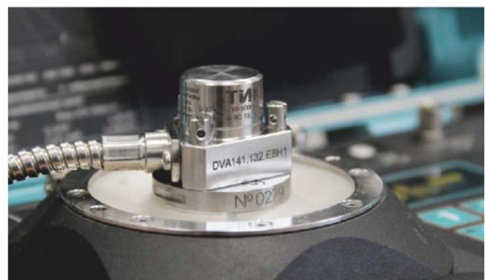
Equipment Testing Department, DVA series vibrodiagnostic sensor tests
