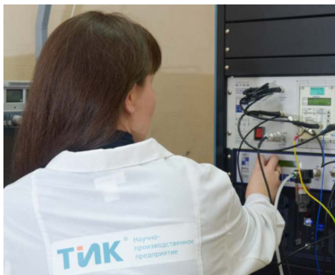
Calibrating the vibration sensors
