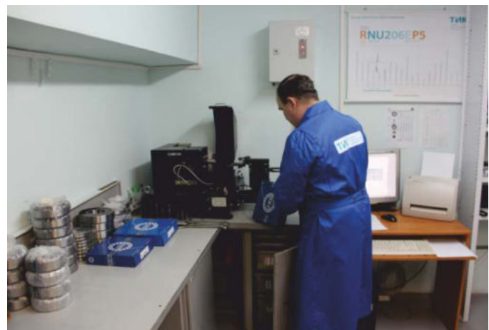
Diagnostics of ZKL bearings on the SVK-A Vibration Control Stand in the Laboratory TIK-2 area
